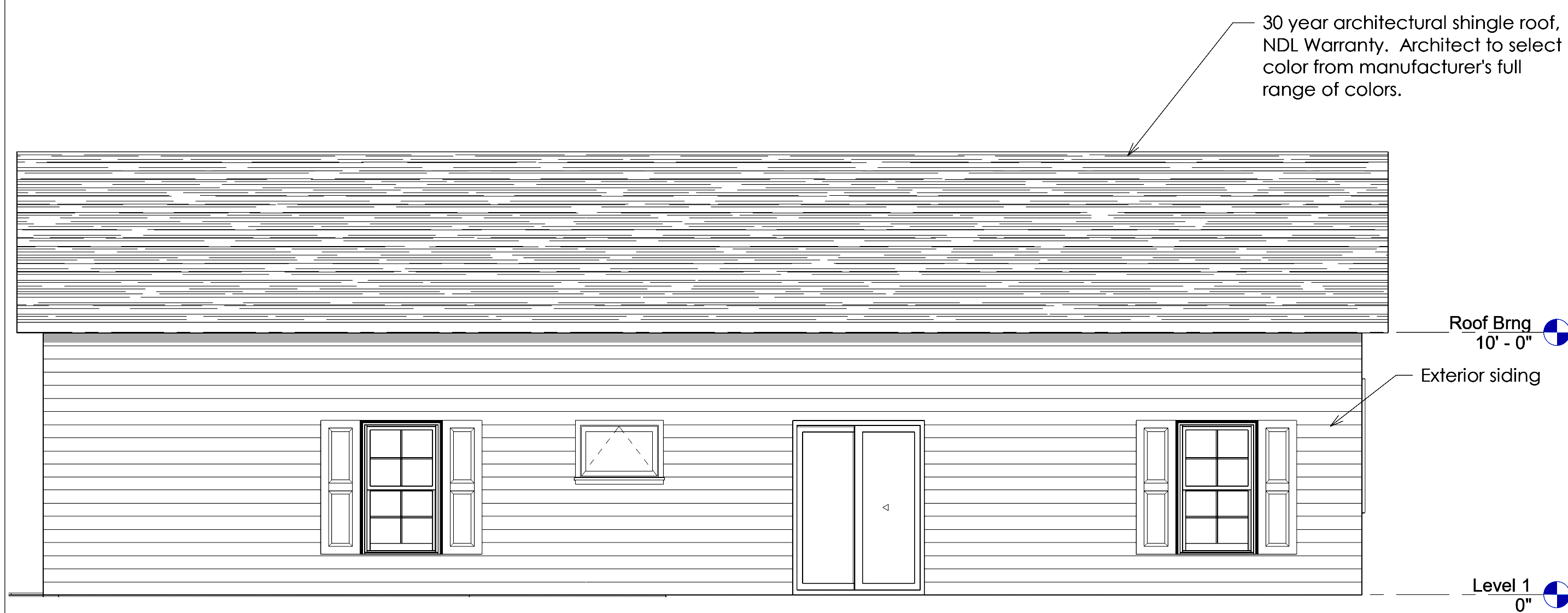
E1 East Elevation V-3 1/4" = 1'-0"
